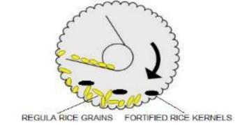
Figure: Principle of Blending inside the Rice Length Grader
