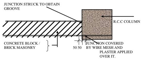
Ceiling plaster shall be done, with a trowel cut at its junction with wall plaster. Similarly trowel cut shall be adopted between adjacent surfaces where discontinuity of the background exists.
